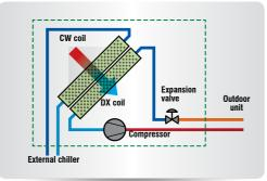
The Dual Cooling version houses - in addition to the direct expansion evaporating coil and in series with respect to the air flow - a chilled water coil that can, for example, be fed by a chiller. This means that the required cooling capacity can be supplied even when there is a fault on the main refrigerating circuit, thus ensuring maximised system redundancy.
