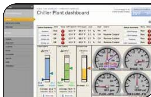
Tracer SC dashboard uses an easy-to-interpret, graphical display to report current operating conditions and energy usage.
